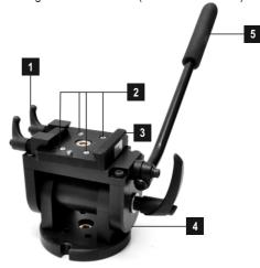
Slide AK-101 sliding plate into AKC-3 adapter base mounted on the head and lock the clamps [3]. You can remove the head handle for a more convenient assembly. Before you insert crane mounting plate into the adapter base it is crucial that the adjustment knob [1] is maximally unscrewed. Use the adjustment knob to level the arm of the crane.
