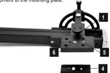
Insert Manfrotto 501PL mounting plate into Manfrotto MN577 adapter mounted on HG-2 head. Next, by screwing the adjustment knob level the arm of the crane.
