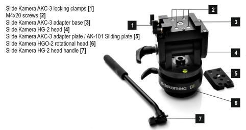
Slide the AKC-3 adapter plate into its base mounted on the head and lock the clamps. You can remove the head handle for a more convenient assembly. Before you insert crane mounting plate on the adapter base it is crucial that the adjustment knob is maximally unscrewed. Use the adjustment knob to level the arm of the crane.
