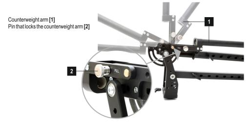
After mounting the accessories on the mounting plate of the crane balance the crane by mounting the weights on the arm. Please remember that maximum permissible counterweight is 6kg for 4.5kg of payload on the crane mounting plate. Once you balance the crane properly tighten the safety nuts. The counterweight arm is also equipped with a sliding weight (used mainly when lens changing) that allows to balance the crane without the need of adding additional counterweights.
