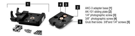
Mount Slide Kamera AKC-3 adapter base to HST-2 or HST-3 tripod socket using Manfrotto half ball. Mount Slide Kamera AK-101 sliding plate to crane rotational head using Slide Kamera 1/4" and 3/8" photographic screws. Unlock AKC-3 adapter clamping levers, slide AK-101 sliding plate (mounted to ROAD JIB rotational head) into AKC-3 adapter base, thus connecting Slide Kamera ROAD JIB camera crane with Slide Kamera HST series tripod. Remember to lock the clamping levers.
