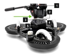
M4 holes spacing allows also for mounting Manfrotto MN577 adapter with MN501PL sliding plate on the low base of HSO-4 rotational slider. Method of mounting is the same as in case of mounting AKC-3 adapter.
