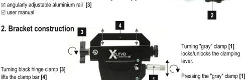
shifts the clamping lever [2].
